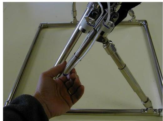
Step 4: To find the correct position for the hinge in the strut, fold the frame (in this case a bimini) back onto its aft legs. For boats with a backstay passing through the bimini fabric, fold all bimini frames up to the backstay and secure. Pull the slack patterning line down alongside the folded frame and mark the very bottom. *Incorrect hinge placement will result in a folded strut that binds up or folds out of position.*
