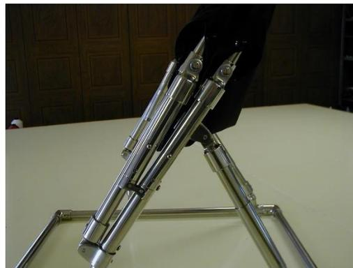
Step 1: Struts can be placed inboard or outboard of the frame. Place the struts as high as possible for the most powerful leverage. See installed strut in locked and folded positions above.
